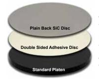
Double sided adhesive discs are adhered to a standard platen and used to secure plain back silicon carbide abrasive discs. Each provides 25-75 disc pulls depending on grit size, cycle time and force.
